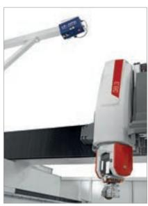
The optional laser projector guides the machine operator during the placement of the suction cups, thus making the table preparation easier and faster.
