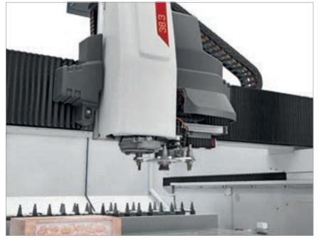
8-position revolver storage on the fly to reduce the passive time for the most frequently used tools.
